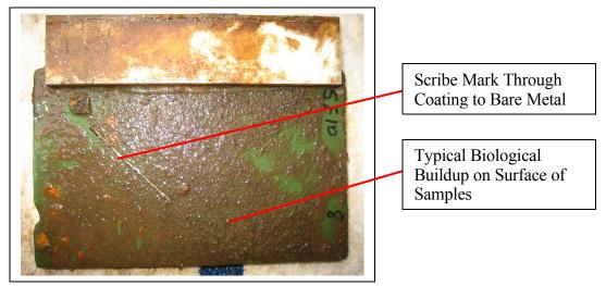
Figure 3. Coated Test Coupon
