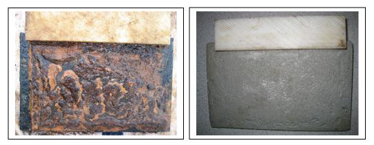
Figure 2. Uncoated Test Coupon Before and After Cleaning
