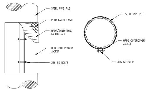
Figure 7. HPDE Pipe Pile Protective System
