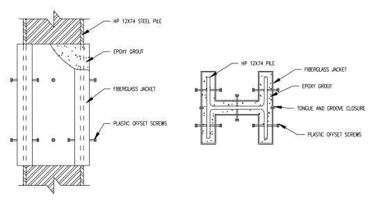
Figure 6. H-Shaped Fiberglass Protective System
