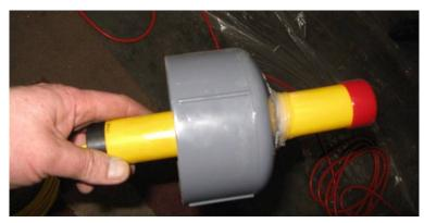
The reference electrodes (shown with protective red cap) were inserted through holes in the bottom pipe caps of samples, glued to caps, and sealed.
