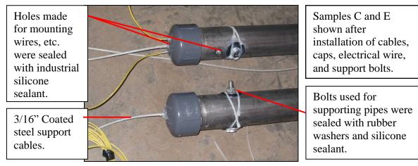
Picture 20: Pipe Sample Sealing
