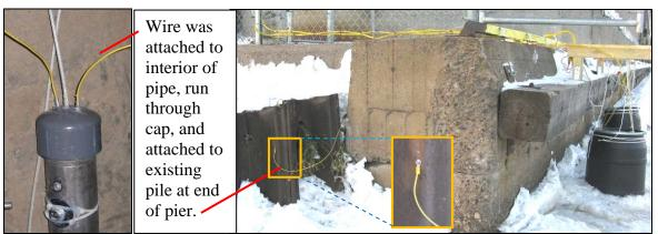
Pictures 24 & 25: Sample C Attached to Existing Sheet Pile
