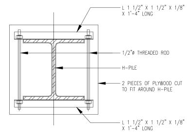
Figure 3: Series 500 H-Jacket Base Plate Detail
