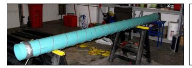
10' long 6" diameter PVC pipes were wrapped in self regulating electric heated cord typically used for rain gutter de-icing. Each cord has 300 watts capacity.
