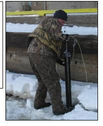
Sample D shown being lowered through hole in ice along pier.
