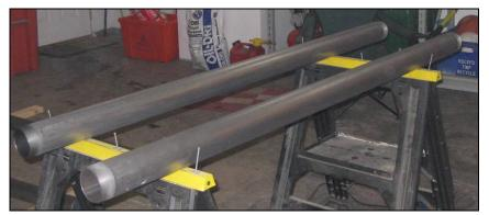
Test samples shown after sandblasting and prior to installation of coating, wires, and hardware.
