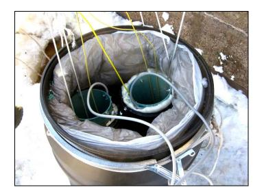
The PVC pipes were then lowered through holes in the ice and supported such that their tops were ~30" above the ice surface. Insulated plastic barrels were then placed around the two pipes to prevent holes from freezing. Batted fiberglass insulation was placed in the top of each 6" pipe for further insulation (not shown in picture).
