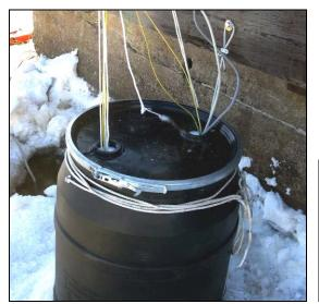
Each barrel cover was insulated for further freeze protection. The covers can be removed to allow pipes & anodes to be removed and inspected during winter months as well as allowing water conductivity measurements.
